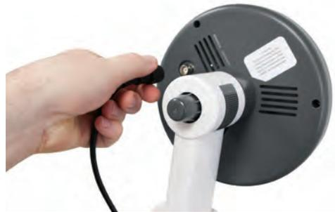
**Figure 2. Connecting Coaxial Cable to Monode Drum**
