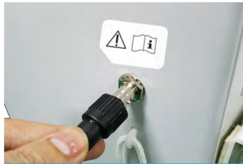
**Figure 2. Connecting Coaxial Cable to the Cart**
